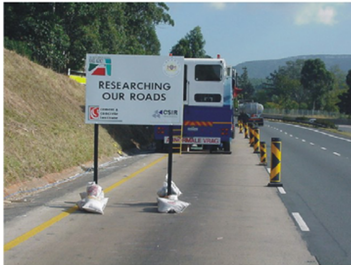
◀ HVS testing on the N3 PCC inlay
