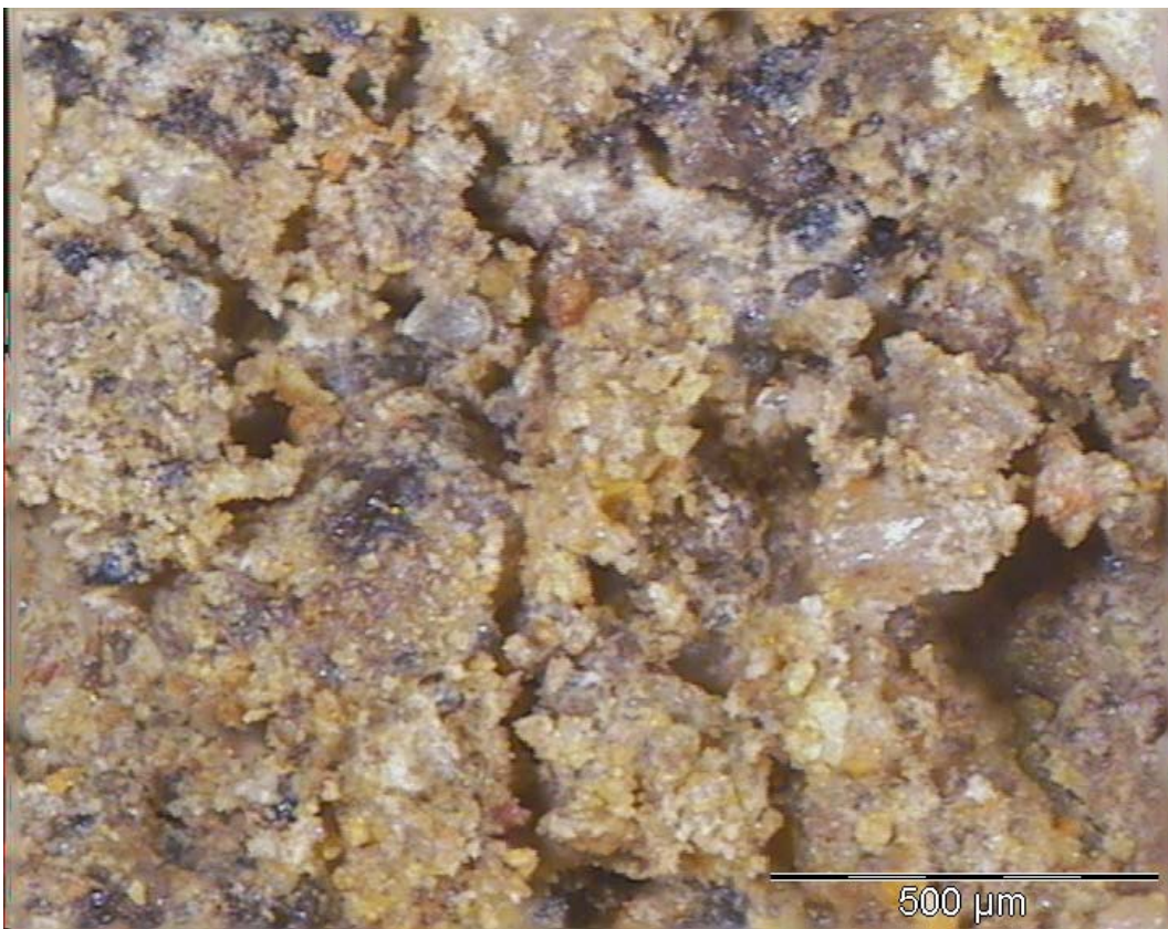
Photograph A8. 1.8% net bitumen, 1% cement, 40x magnification
