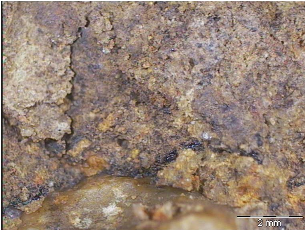
Photograph A17. 3.0% net bitumen, 1% cement, 7x magnification (note bitumen film around bigger aggregate)
