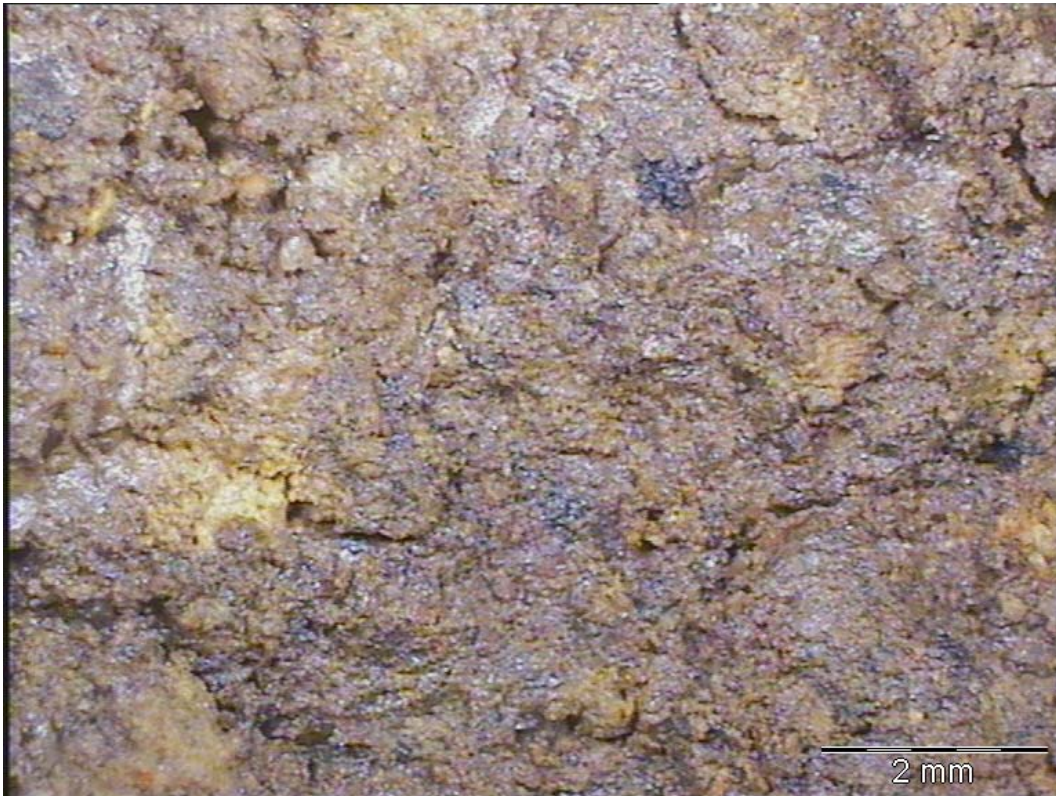
Photograph A5. 1.8% net bitumen, 0% cement, 7x magnification
