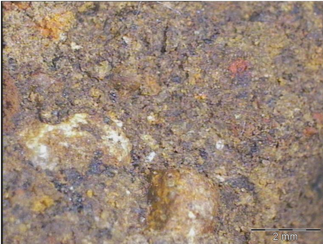
Photograph A15. 3.0% net bitumen, 1% cement, 7x magnification
