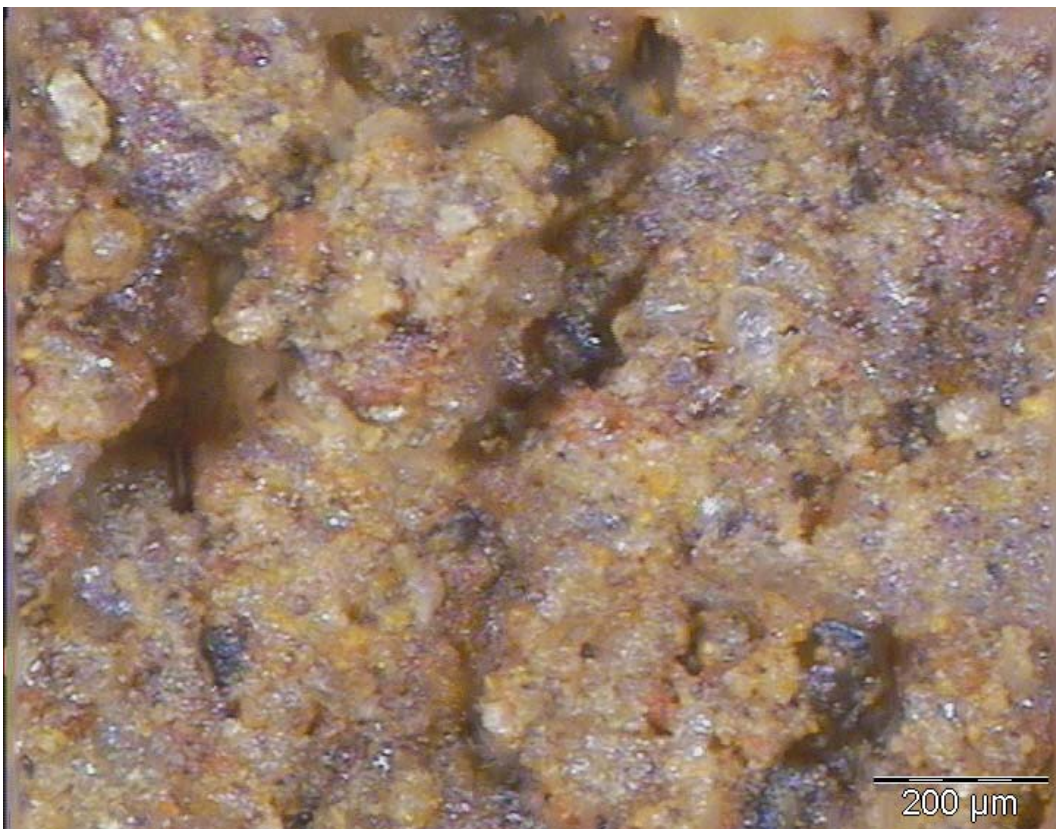
Photograph A2. 0.6% net bitumen, 0% cement, 50x magnification
