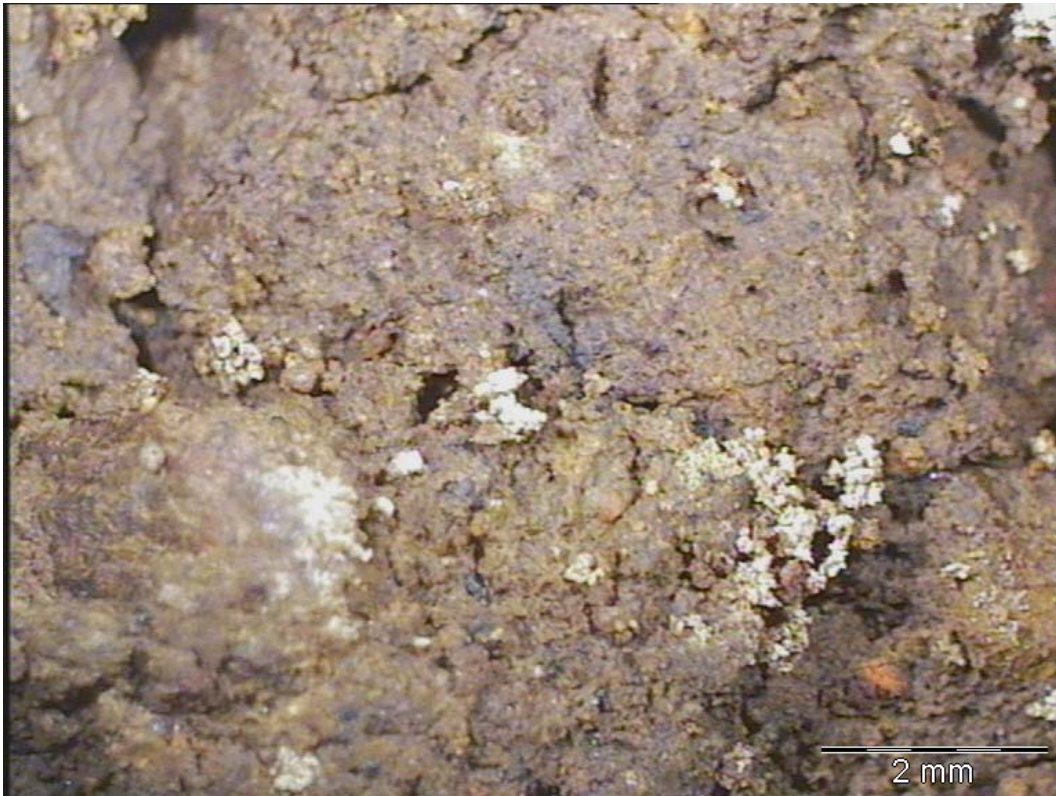
Photograph A1. 0.6% net bitumen, 0% cement, 7x magnification
