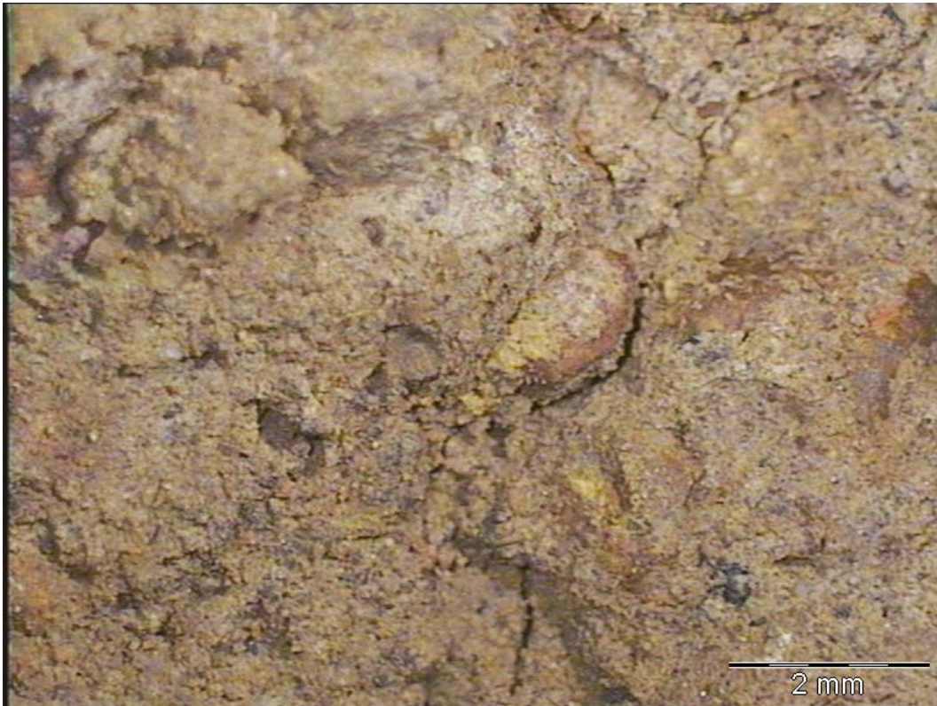
Photograph A3. 0.6% emulsion, 1% cement, 7x magnification
