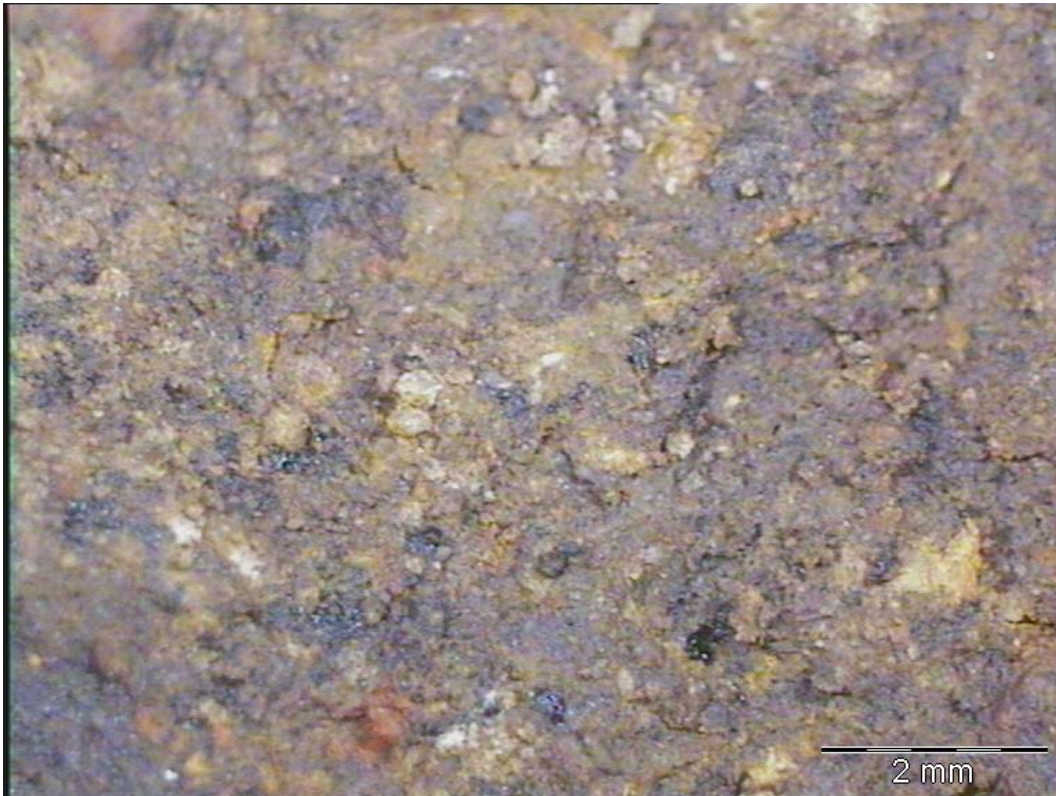
Photograph A13. 3.0% net bitumen, 0% cement, 7x magnification
