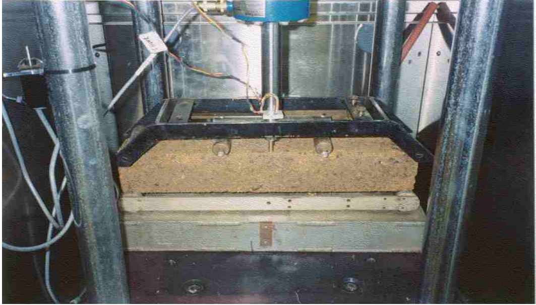
Figure 8. Test Setup of Flexural Beam Test
