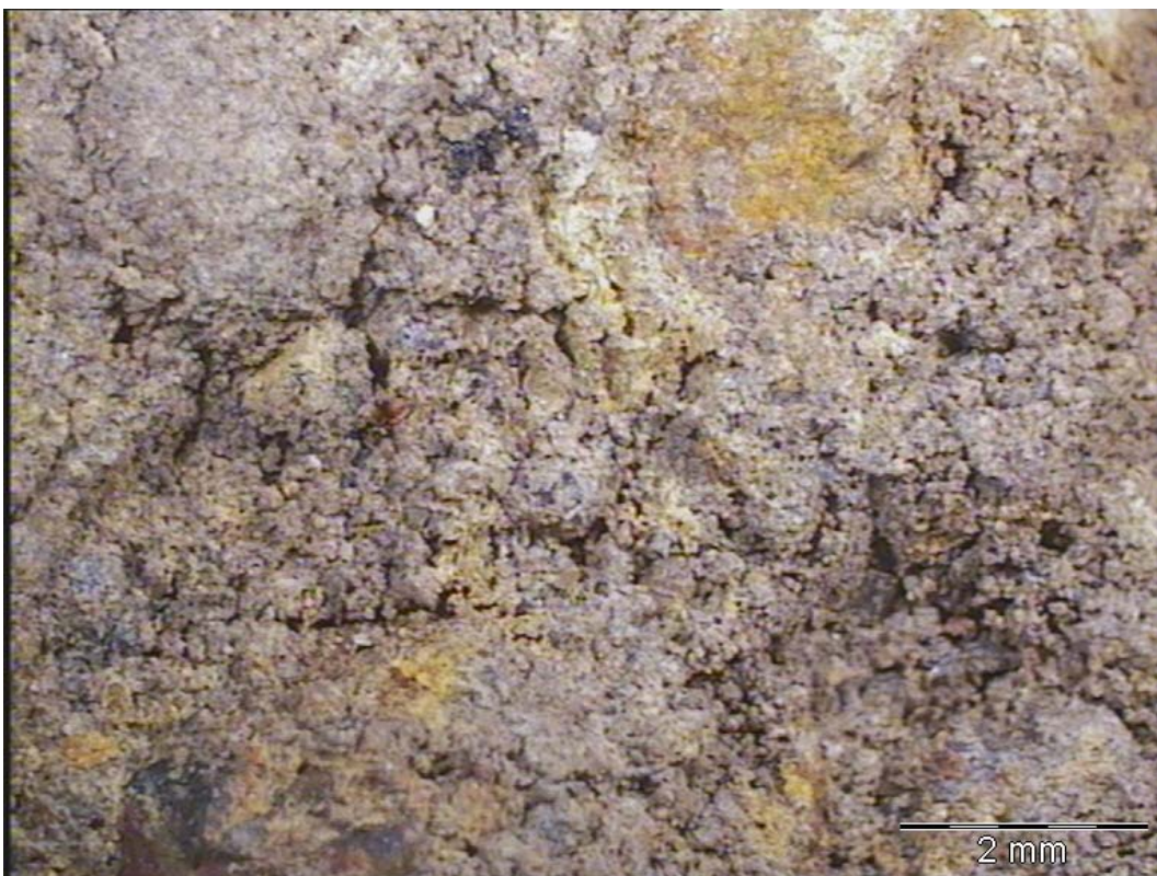
Photograph A10. 1.8% net bitumen, 2% cement, 7x magnification
