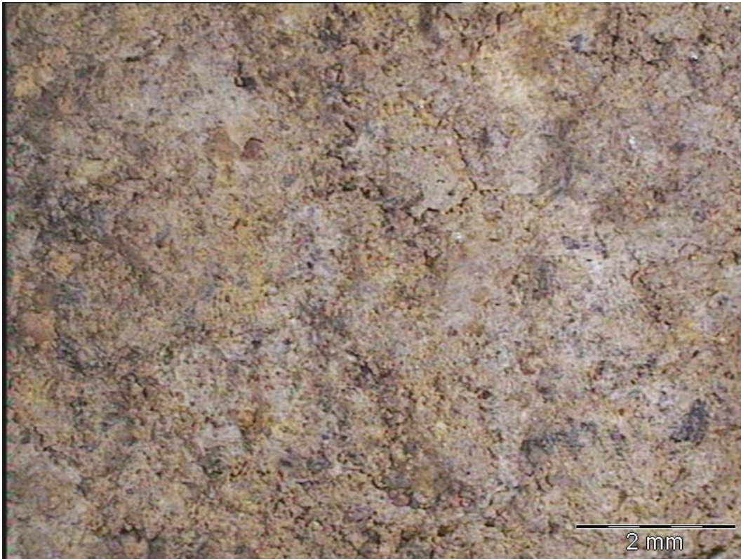
Photograph A7. 1.8% net bitumen, 1% cement, 7x magnification
