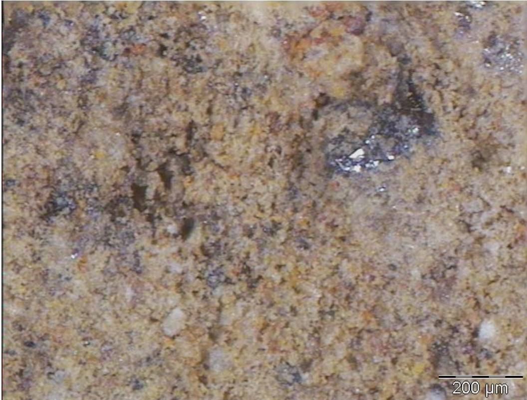
Photograph A9. 1.8% net bitumen, 1% cement, 50x magnification
