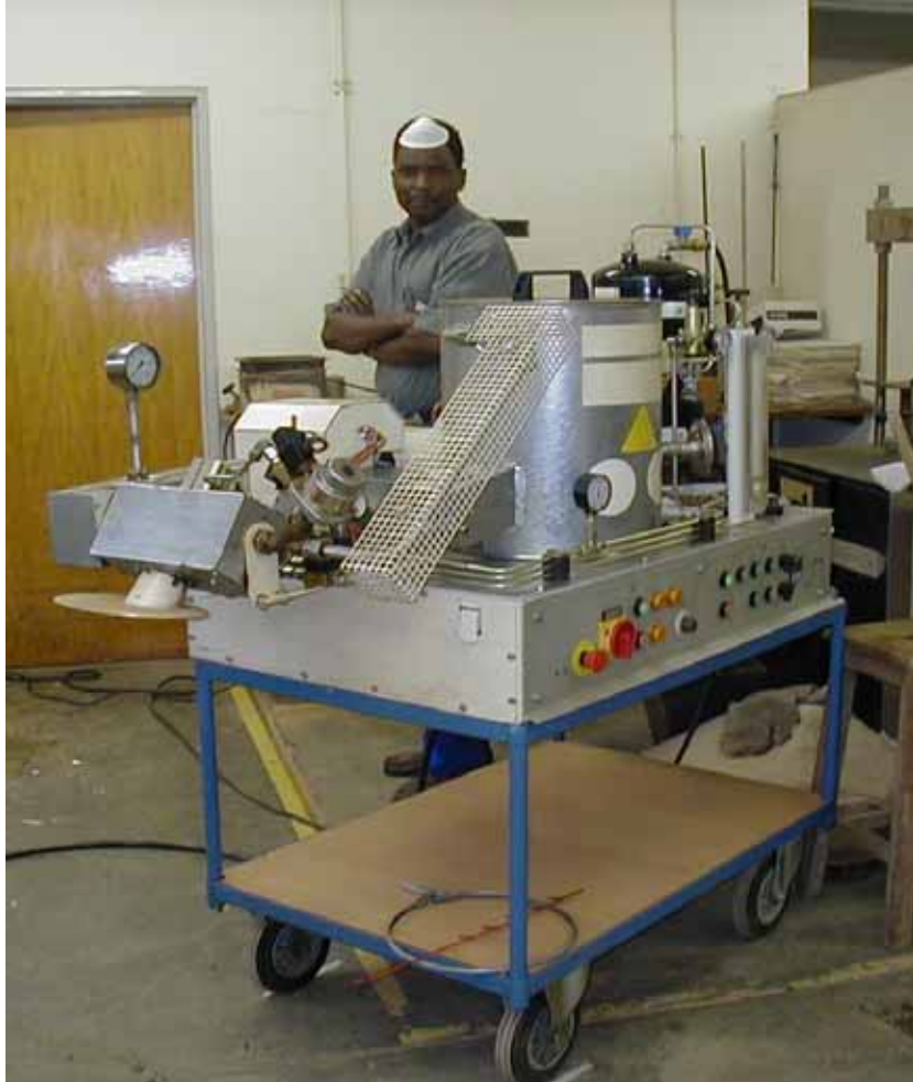
Figure 2. Wirtgen Foaming Apparatus
