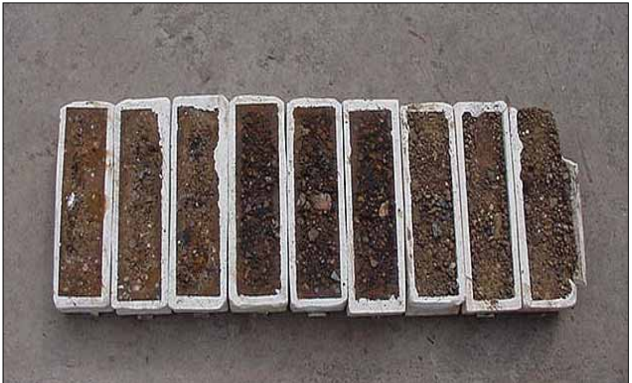
Figure 4. Erosion Specimens Treated with Foamed Bitumen
