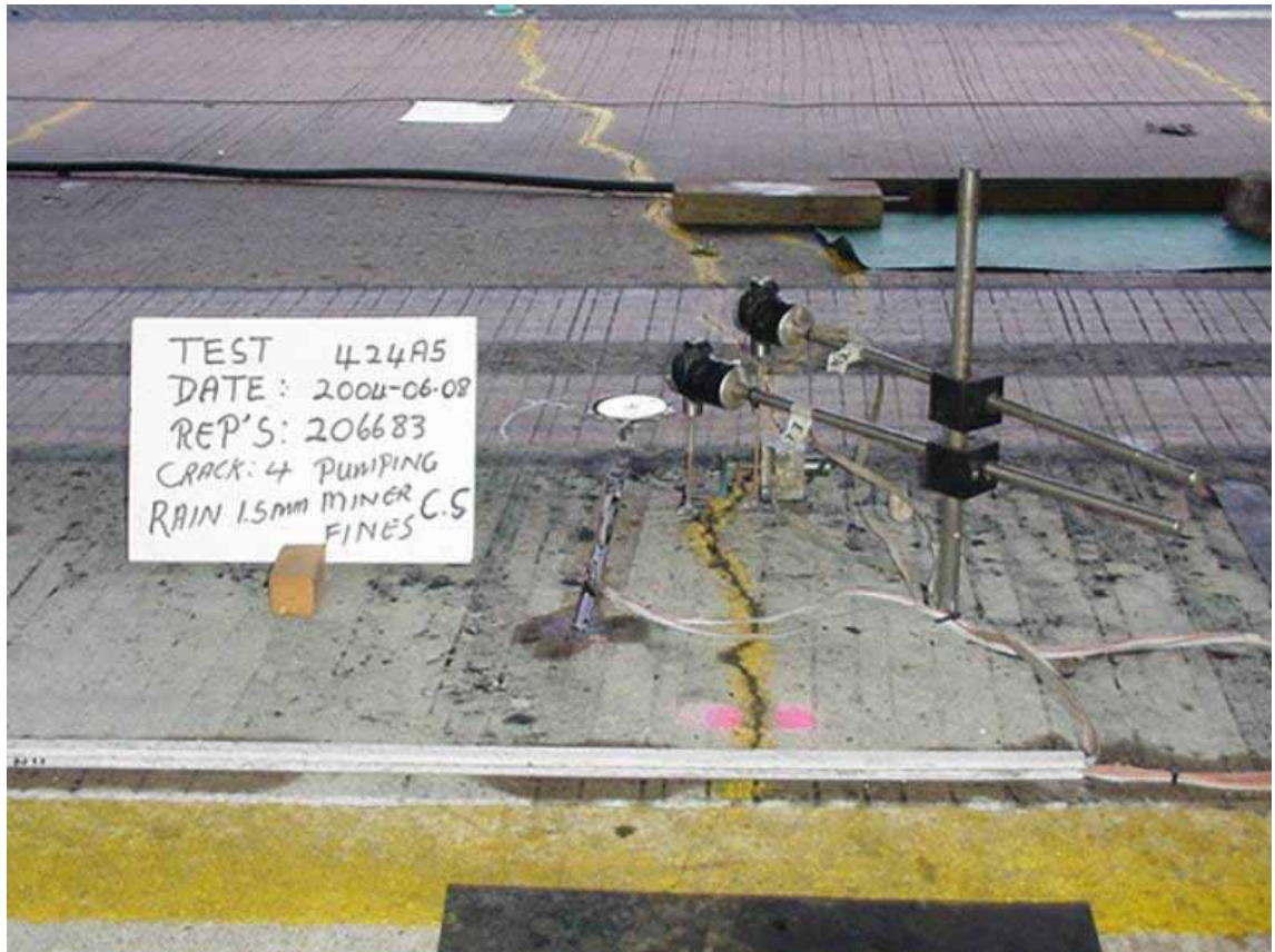
Picture 5.5: Pumping of fines after 206 683 repetitions
