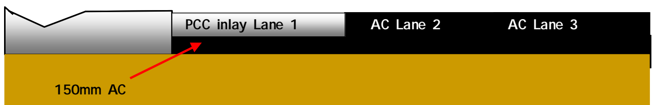
Figure 5.8: Expected pavement structure at km 16.3
