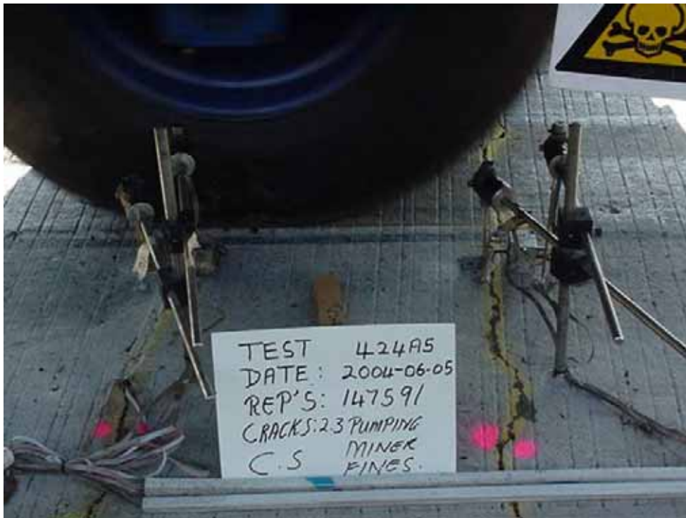
Picture 5.1: Minor degree of pumping after water has been added
