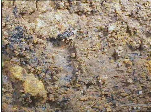
Figure 5. Sample from Laboratory (5 per cent bitumen)
