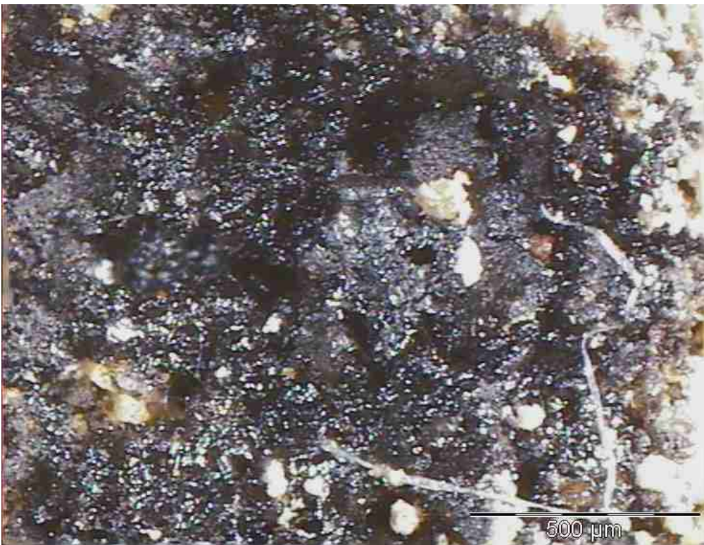
Laboratory mix: 1.8% foamed bitumen, 2% cement. Small film of bitumen (thicker than on HVS material)
