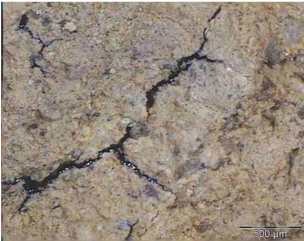
Laboratory mix: 3% foamed bitumen, 1% cement. Channel of bitumen in the mix
