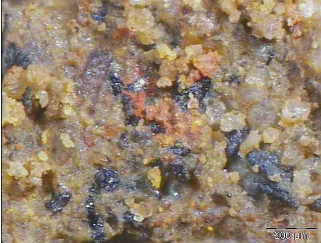
Laboratory mix: 5% foamed bitumen, 1% cement. Small 'balls' of bitumen.
