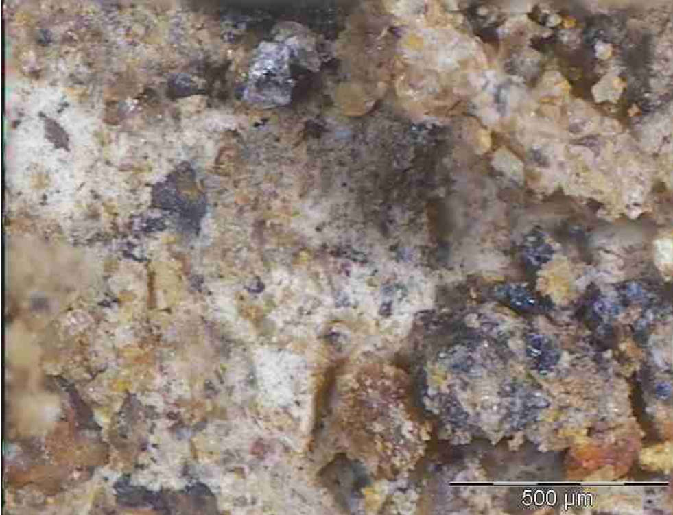
Laboratory mix: 1.8 % foamed bitumen, 2% cement. Possible forming of cement bonding (light colour)
