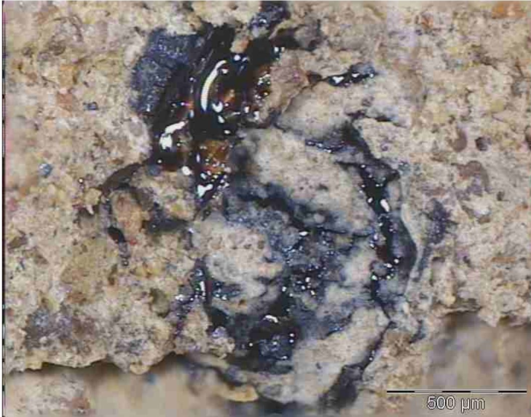
Laboratory mix: 3% foamed bitumen, 1% cement. Bitumen mixed with aggregate
