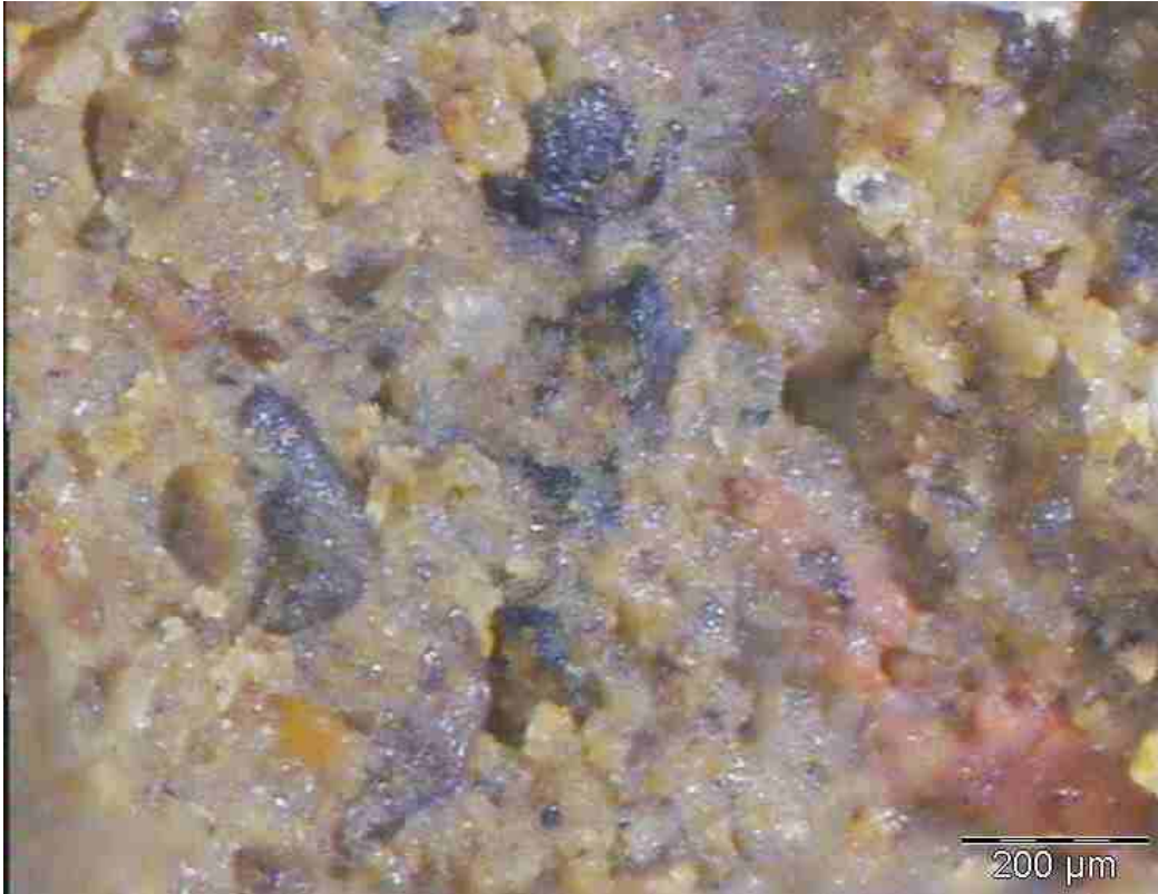
Laboratory mix: 1.8% foamed bitumen, 1% cement. Small 'balls' of bitumen.
