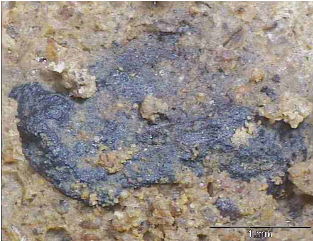
Laboratory mix: 3% bitumen, 1% cement. Possibly an piece of the old surface seal.
