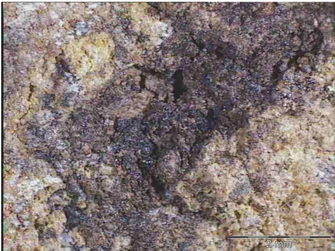
HVS mix. 1.8% foamed bitumen, 2% cement. spray of bitumen on the aggregate
