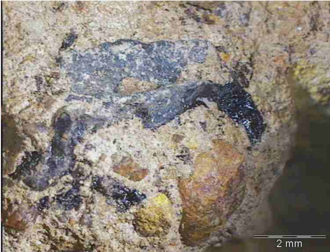
HVS mix. 1.8% foamed bitumen, 2% cement
