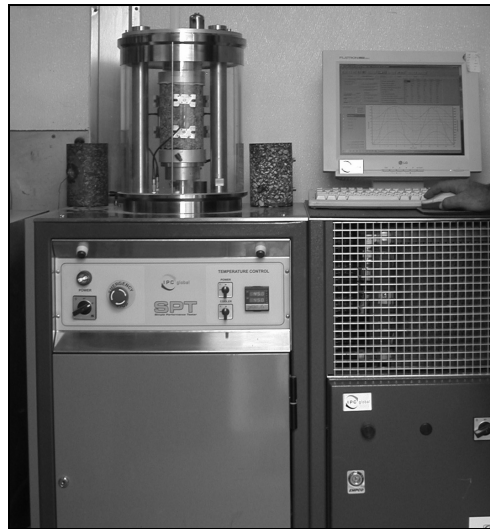
Figure 1. Simple Performance Test (SPT) Device in FHWA Mobile Asphalt Laboratory
