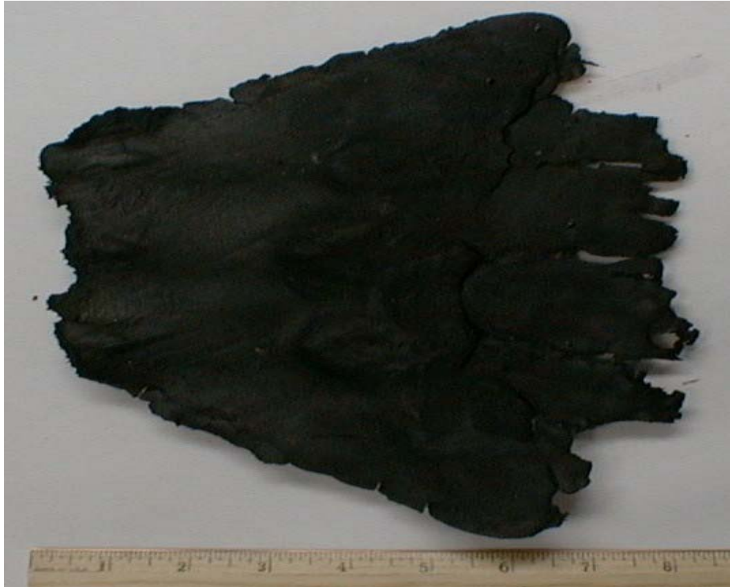
FIGURE 4 A photographic illustration of rubber build up removed from a test section.
